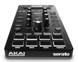
The Akai Pro AFX, an example of a modular DJ controller that can be added to a DJ system to do a specific task.
